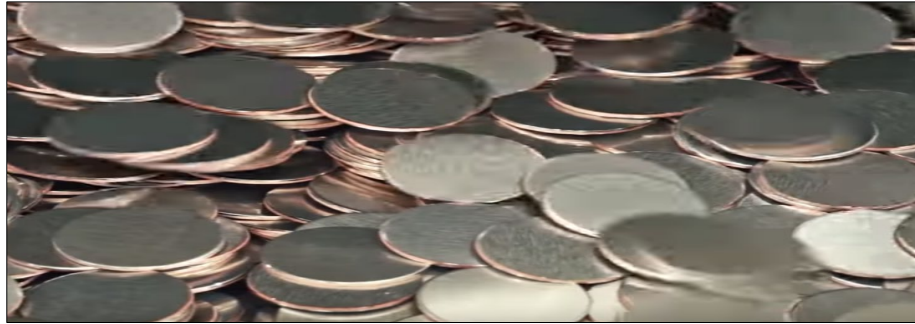
Figure 2: Blanks Punched Out of a Raw Material Coil
