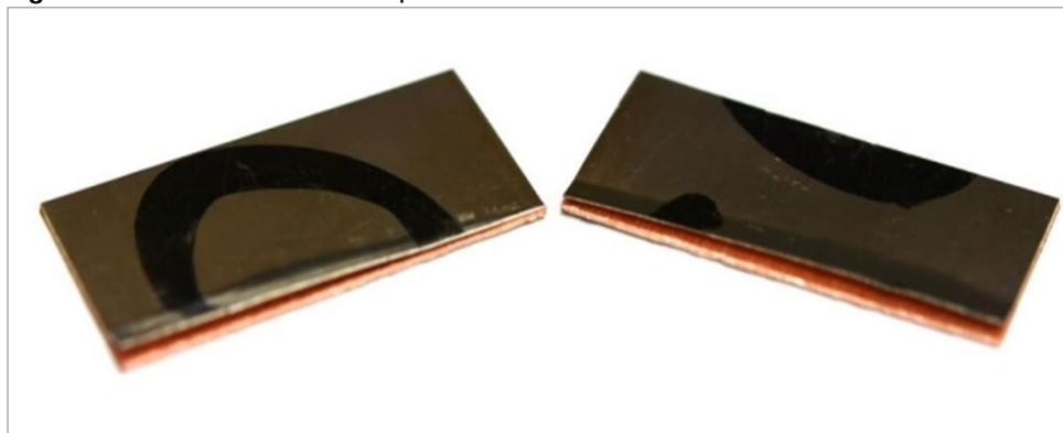
Figure 5: A Delaminated Coupon
