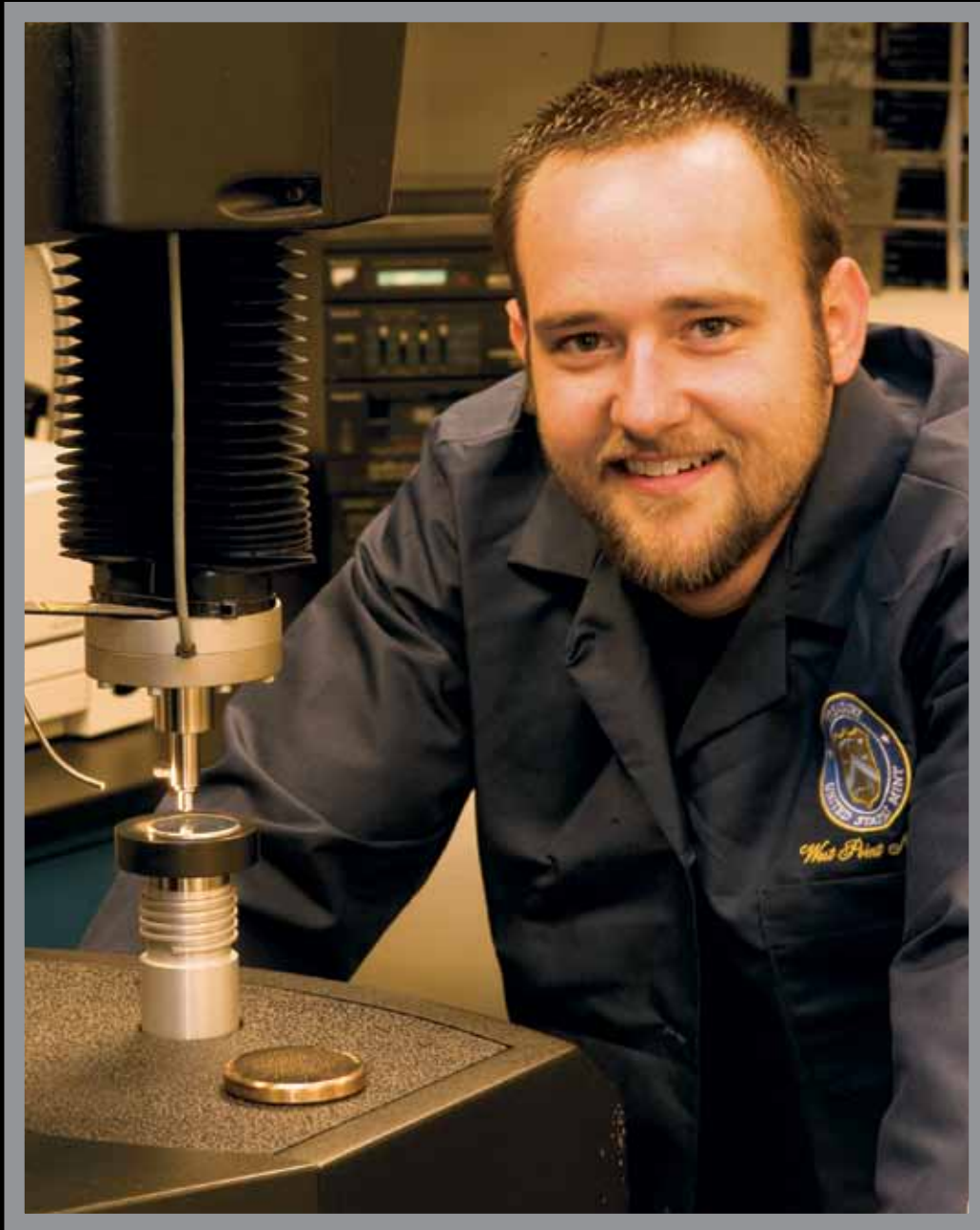
United States Mint at West Point employee Keith Gopel checks the hardness of silver blanks. The United States Mint has established specifications for hardness, so employees must test incoming blank shipments to make sure they meet the criteria.
